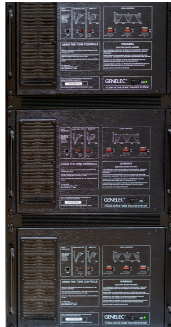
▲ One of the Genelec 1034B Studio Monitors used for LCR positions behind the screen. ▼ The rack-mounted amplification for the Genelec speakers is kept in ventilated cupboards outside the main theatre, easily accessible for maintenance.
