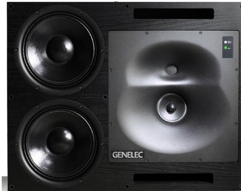
▲ One of the Genelec 1034B Studio Monitors used for LCR positions behind the screen. ▼ The rack-mounted amplification for the Genelec speakers is kept in ventilated cupboards outside the main theatre, easily accessible for maintenance.
