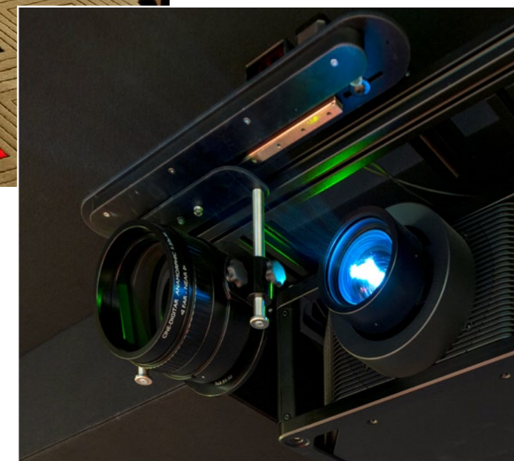
◀ MAIN IMAGE: The finished home cinema with 212-inch screen; ▲ ABOVE: The Sony native 4K projector fitted with automated Schneider Kreuznach anamorphic lens and custom lens-sled.
